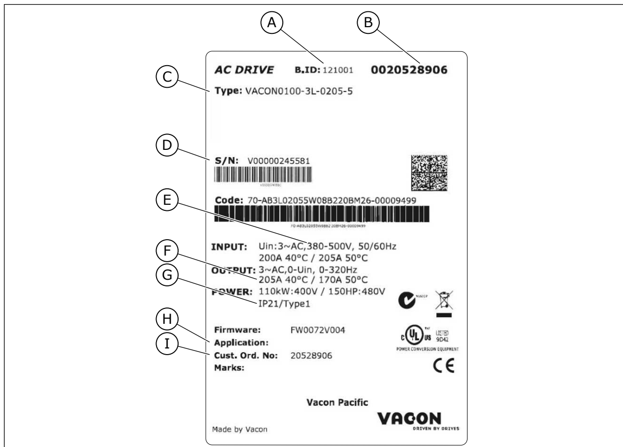
Fig. 1: The package label of Vacon AC drives
